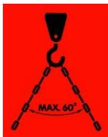
**Warning !** Use all **four** lifting eyes or use lifting tool as supplied by Tolsma Tankbouw.
