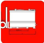
Some models are equipped with it a guide for forklift spoons. Moving an IBC with a forklift must only be done on flat terrain.
